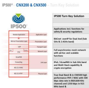
Figure 5. IP500® uses a finer subdivision of the data link layer than the previously known OSI model. (Image: IP500® Alliance)
