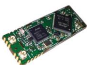
Figure 2. The IP500® Wireless module CNX200 contains a microcontroller for the IP500® network stack and also the antenna. It fulfills all requirements for worldwide certification
